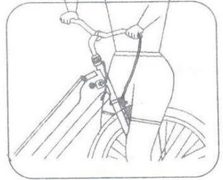
Some models have a light console that attaches to the handlebar. Attach this with the plastic brackets and screws provided.
