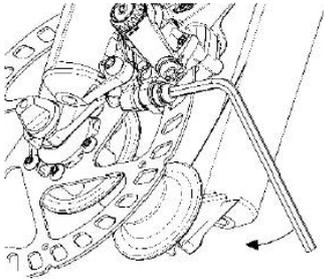
Always check that both your front and rear brakes are properly adjusted before riding your bike. Squeeze your brake together and slip the cable into the through. You may need to adjust the cable length by loosening the nut and sliding the cable through to the proper position. Retighten the nut to hold the proper position.
