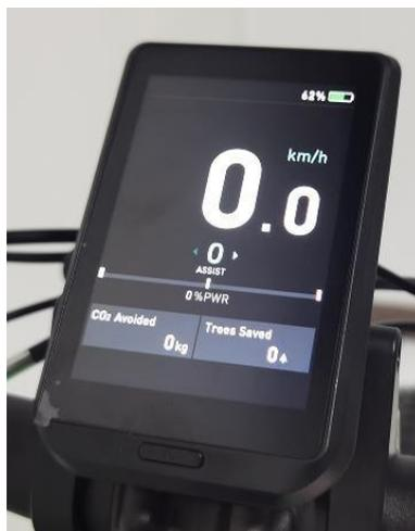
Long press the “
